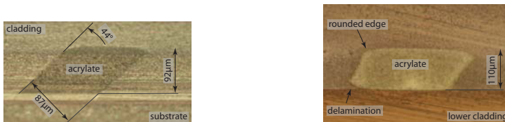
Figure 7.4: Cross-section of tilted acrylate micro-structures on a polyimide substrate ( left ) and on a lower PU-cladding ( right ), both are patterned using the tilted laser-head. The acrylate structure on the lower cladding shows delamination ( right ).
