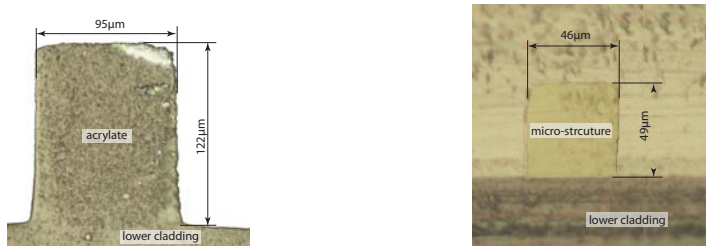
Figure 7.3: Cross-section micrographs of in-plane micro-mirrors on lower cladding, showing vertical sidewalls of over 120 µm in height, with only a small inclination on the bottom part of the structure (exposed by a laser-diode based vertical laser-head) ( left ), micro-structure with about 50 µm cross-sectional dimension (exposed using the frequency tripled Nd:YAG laser) ( right ).
